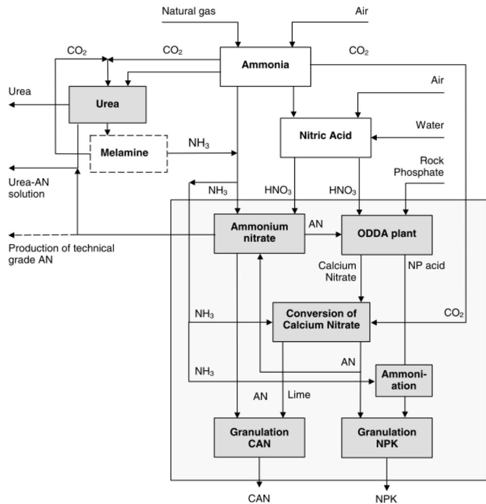
Figure 17: Block diagram of the production of fertilisers (shaded) and of substances used for the production of fertilisers at Agrolinz Melamin GmbH. [24]
