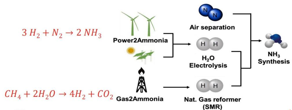
Figure 1: Schematic illustration of new sustainable path for the ammonia production by replacing methane reformer with electrolysis in hydrogen production step. [2]
