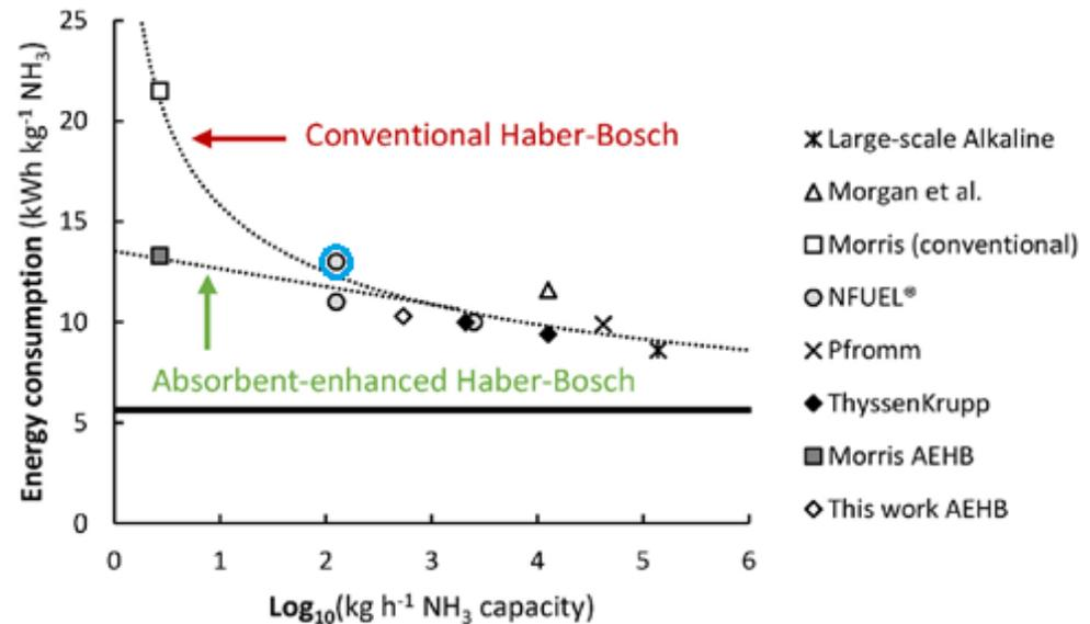
Figure 4: Energy consumption of various electrolysis based Haber-Bosch processes at various ammonia capacity levels (at  $\geq 100$  bar operating pressure for conventional processes, absorbent-enhanced processes are denoted by AEHB). [7]
