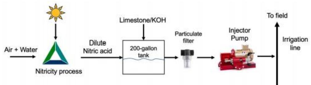
Figure 13: Block diagram showing the integration of the nitric acid generator and irrigation system. [29]
