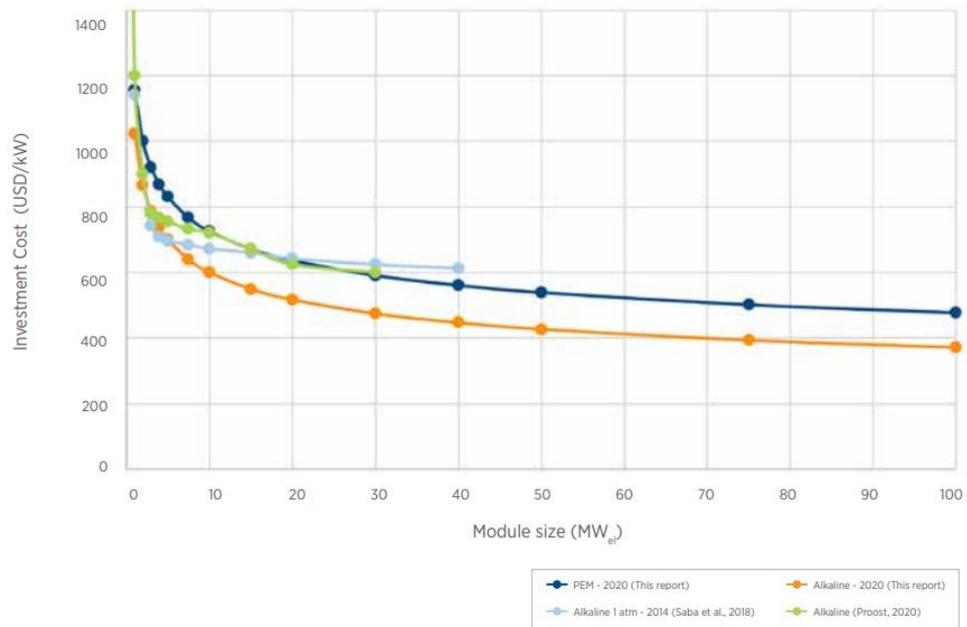
Figure 2: Electrolyser investment cost as a function of module size for various technologies. [8]
