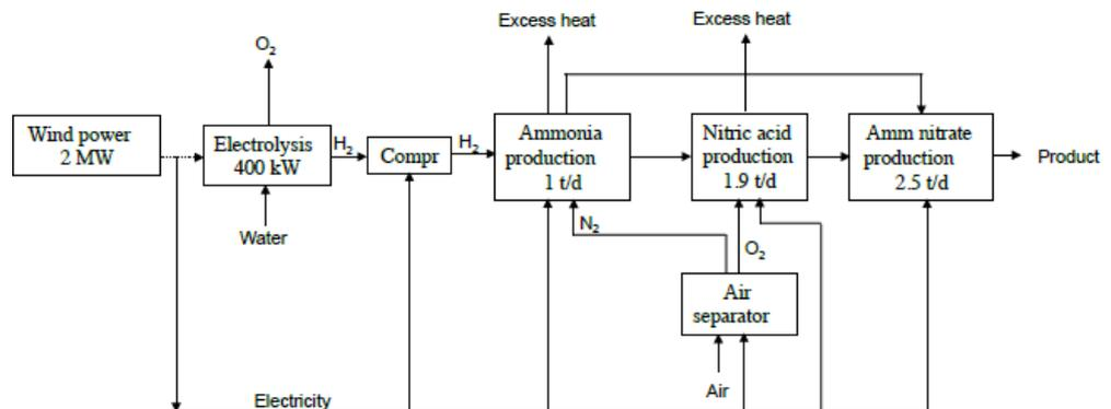
Figure 12: Small-scale ammonium nitrate production process using renewable electricity. [25]
